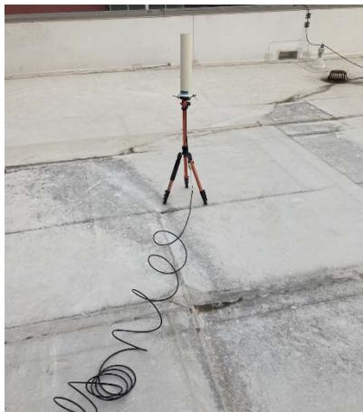
*Figure 1: The Harsh/Synergetics 14A-N omnidirectional antenna mounted on a tripod.*
